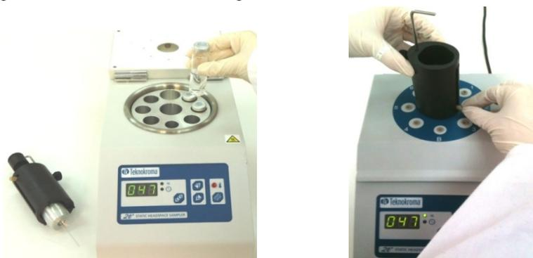
In this situation, we have to show the equilibrium time in the display and press **START** to switch on the chronometer. When the programmed time was elapsed, we press **STOP** and all it's ready to take the gas sample from the vial.
