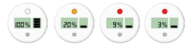
The LED will flash orange when the remaining time of the total lifetime of the device is between 20 and 10 percent.
