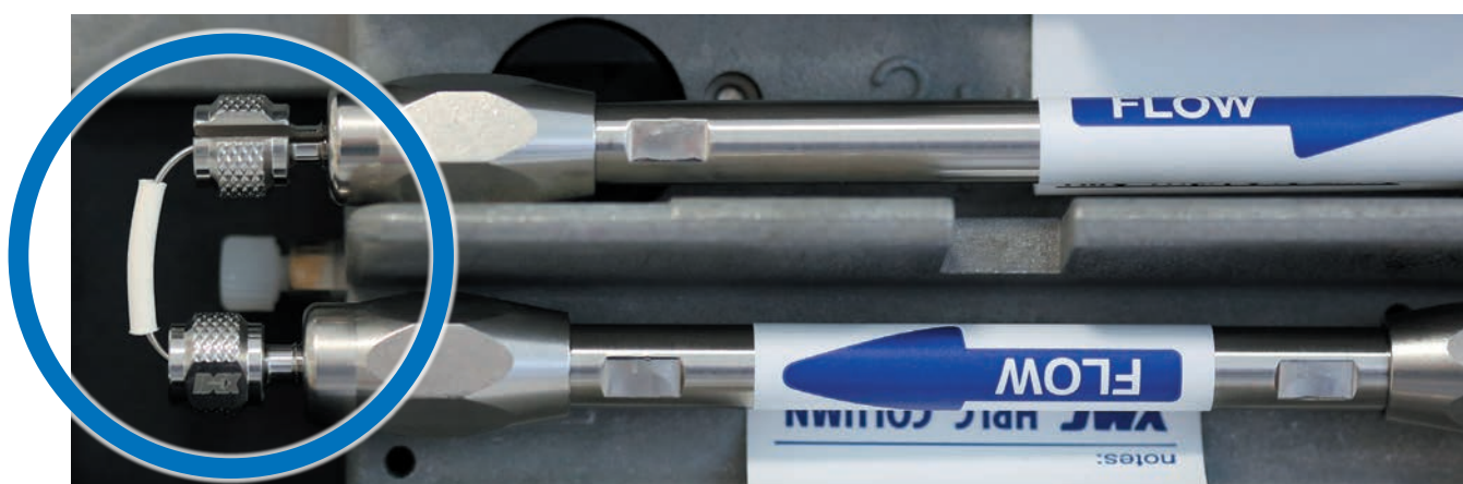
Coupling of two YMC-Triart UHPLC columns using the dead volume free MarvelX™ connector.
