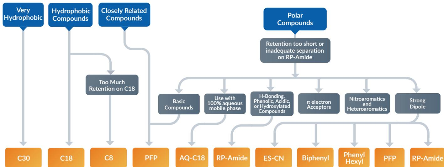
Depending on the nature of the analytes that need to be separated, one can use the flow chart as a guide for choosing the most appropriate HALO® stationary phase.
