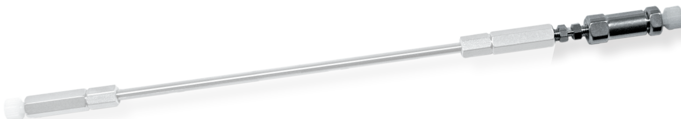
1/32" guard column coupled to a 1/32" analytical column.
