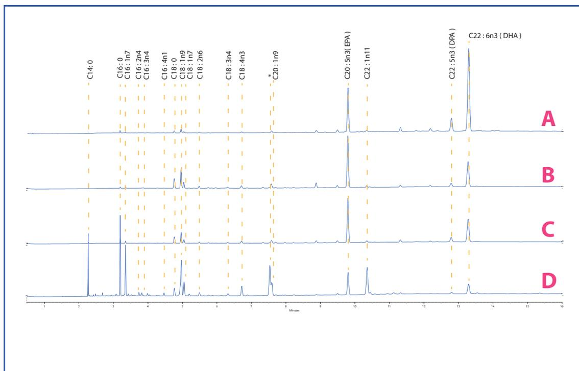
Figure 2. Chromatographic separation of FAME compounds found present in the three omega 3 supplements and the standard fish oil obtained with the **Sapiens-FAMEWAX 20m x 0.18mm x 0.18µm** capillary column. Trace A, B, C correspond to Samples A, B, C respectively and trace D corresponds to PUFA nº 1 standard.
