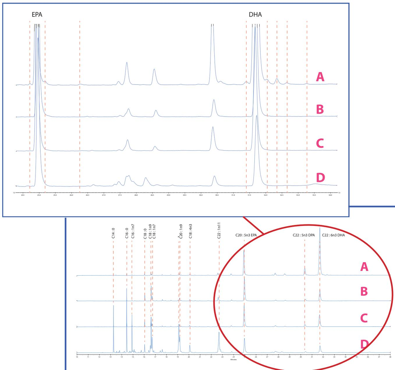
Figure 3. Gas chromatograms of FAME composition of the omega 3 samples and the standard analyzed with the **TR-CN100 75m x 0.18mm x 0.14µm**. Trace A, B, C correspond to Samples A, B, C respectively and trace D corresponds to PUFA nº 1 standard. Zoom of minute 24 to 34, reveals scattered small peaks surrounding EPA and DHA in trace A. These peaks allegedly correspond to *trans*-isomers formed during the processing of fish oil.
