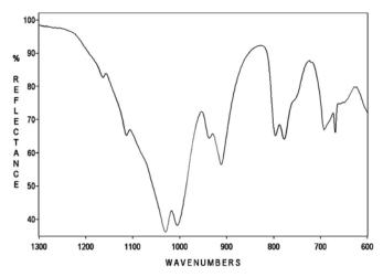
Figure 5. ATR spectrum of 10  $\mu$ m silica powder, recorded at a 45° angle of incidence using the powder sample holder.
