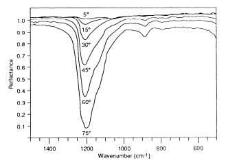
Figure 2. External reflectance of  $0.05 \mu m \, SiO_2$  on aluminum (p-polarization).
