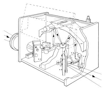
Figure 1. The Seagull™ variable angle reflection accessory.
