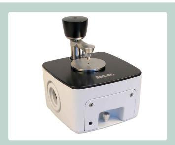
access to the ATR crystal puck. Both plane and pellet anvils are provided with the accessory to allow analysis of samples of various shapes. These anvils are easily interchangeable and stored on the top plate when not in use.
