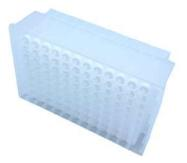
Retention Mechanism: Reverse phase, one of the most hydrophobic phases Functional Group: Polymerically bonded octadecyl C18 endcapped. High Capacity C18 Finisterre OA™ HI B
