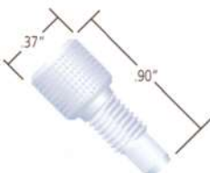
UP-P-100 1/4-28 Kel-F™ Fitting for 1/8" OD tubing Max Pressure 69 bar
