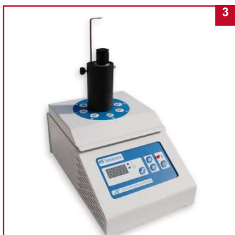
Insert the closed vials with the sample into the heating block.
