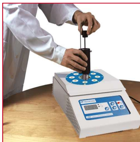
After the equilibrium time is achieved, move the syringe holder into vial number 1, and aspirate the sample by moving the plunger up until the prefixed volume is reached.
