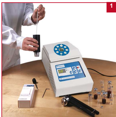
Put the syringe into the black holder.
